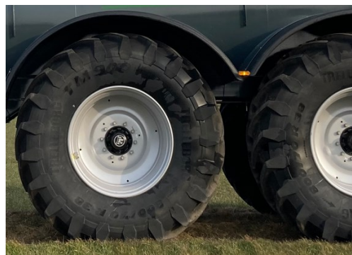
Stor hjulmontering for lav rullemodstand, 800/70 R38 (2050mm).
