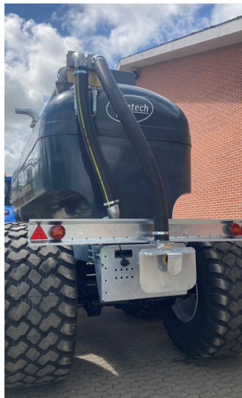
Light board, superspreader and stirring in tank.
