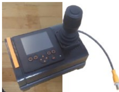
VP Joy Controller for controlling tools.
