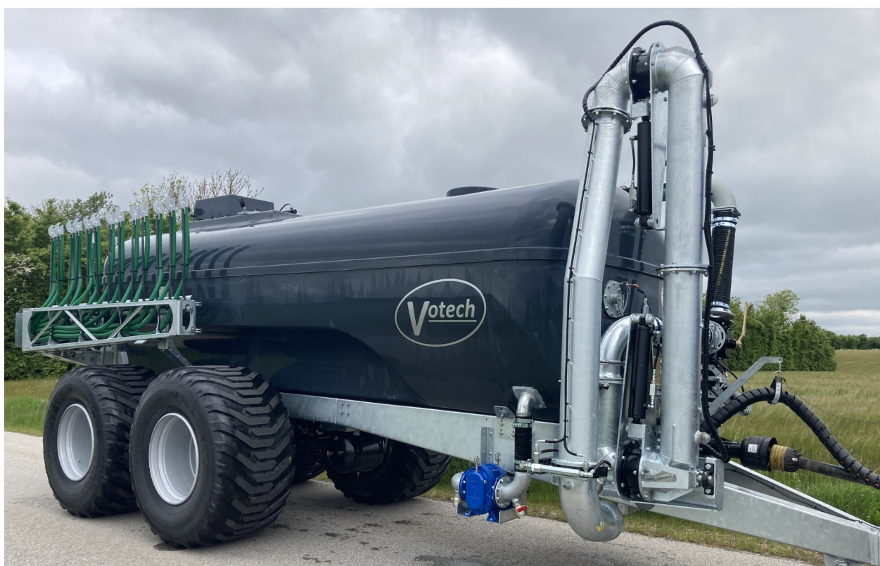
Side loading arm 8", with self-suction.
