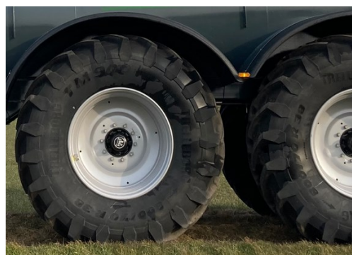
Large wheel fitting for low rolling resistance, 800/70 R38 (2050 mm).
