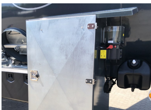
Central lubrication, easy to fill without use of ladder.
