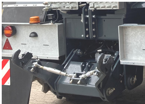
Lift with 8 tonne lifting capacity, fitted so that the implement fits close to the tanker.
