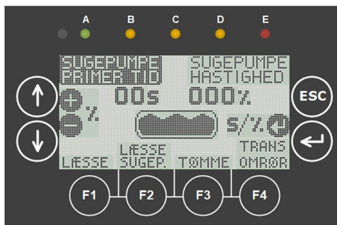
Screen during normal operation. Primer time and speed set here.
