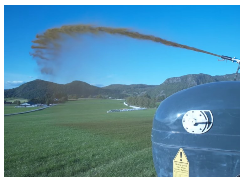
Spreading width up to 60 m, with centrifugal pump.
