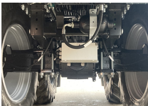
Wheel drive uses tractor's hydraulics. Differential axles, ensuring minimal maintenance.
